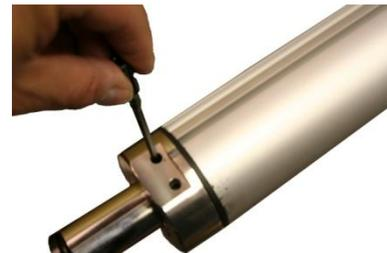
When this is complete, repeat the process with the other screw so that the reel stops when the cover is fully wound onto the reel.
