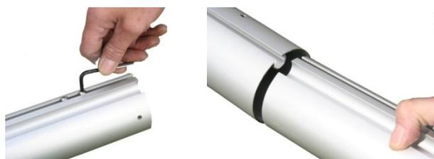
3. When the tubes are connected, and the screws are all connected to the nuts, pull out the tubes evenly to the required width. This should be the pool width plus a minimum of 9" either side. Make sure that the tubes are pulled out evenly either side of the central tube. Tighten the allen screws.
