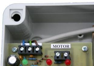
The supply to the motor is connected to the two terminals labeled "motor"
